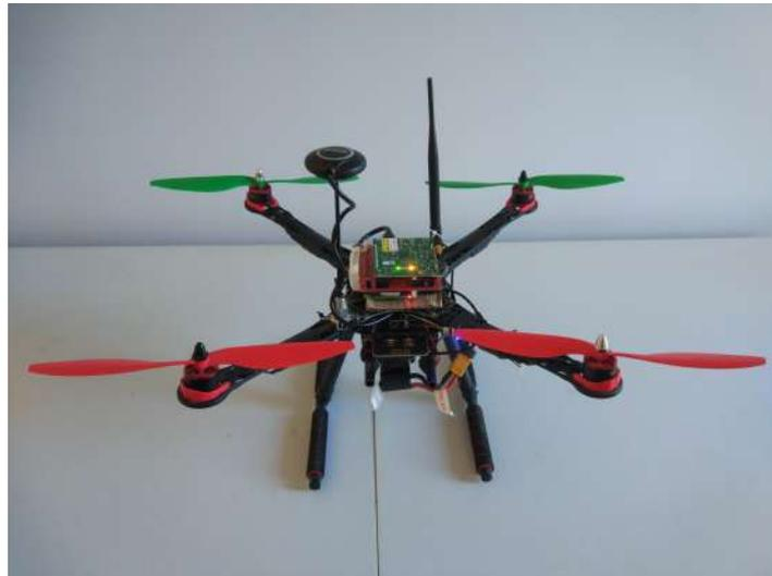
Figure 2. LoRa-drone gateway implementation used for testing
