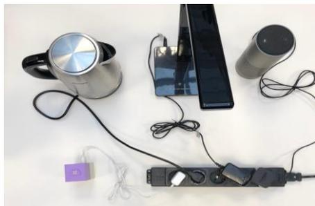
Fig. 7. Devices used in the demonstration. Bottom left: homee gateway, top (left to right): kettle and desk lamp connected to 2 Fibaro Wall Plug, Amazon Echo
